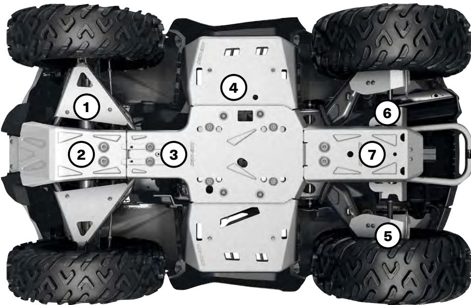
For ultimate durability and strength, all our Aluminum Skid Plates are made with  $\frac{3}{16}$ " (4.5 mm) thick High Strength 5052 H32 Aluminum.
